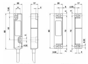
Wide Sensor (Sensor/Actuator) F3S-TGR-NWPR
